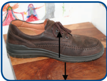
Pairs of contact forces are acting perpendicularly to the contact surface.
